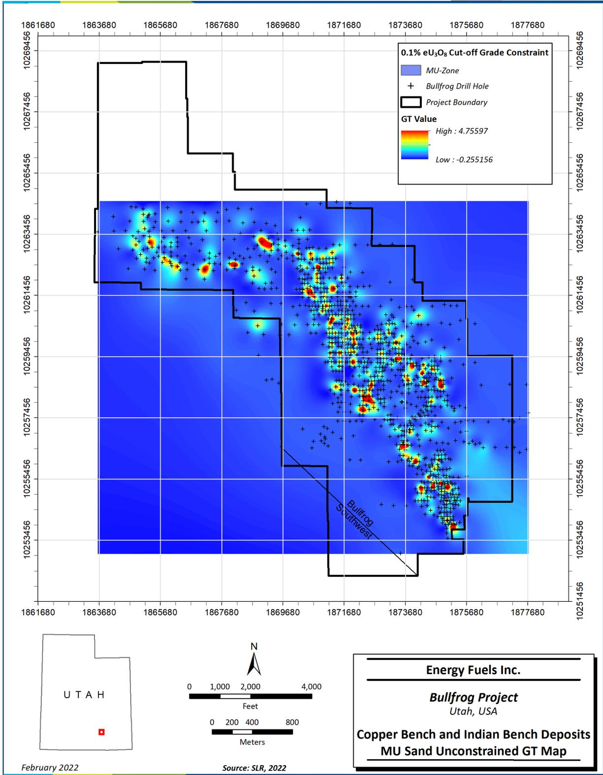
**Figure 14-10: Copper Bench and Indian Bench Deposits MU Sand Unconstrained GT Map**
