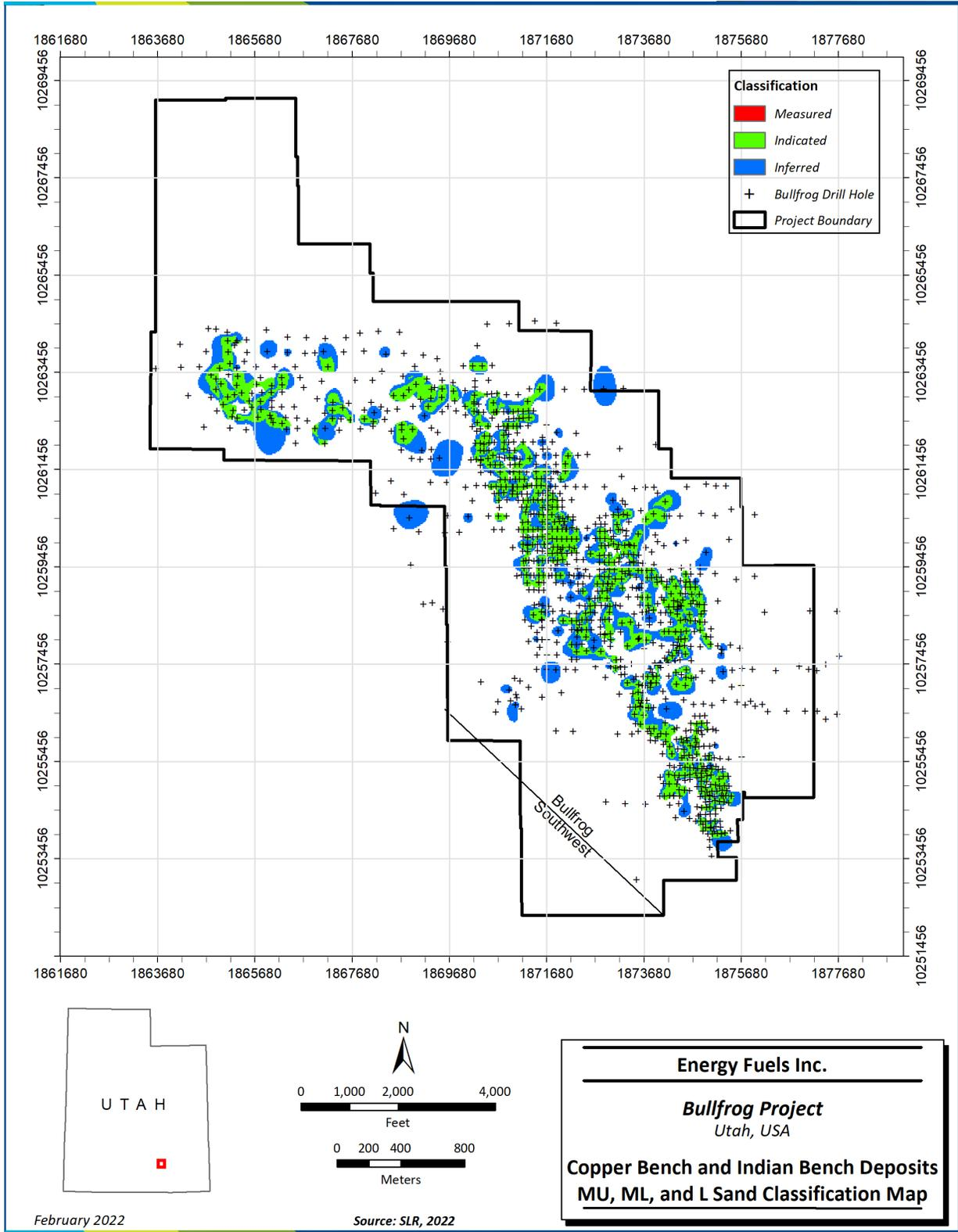
Figure 14-14: Copper Bench and Indian Bench Deposits MU, ML, and L Sand Classification Map
