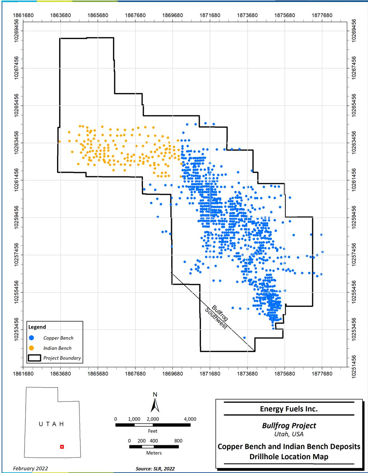
**Figure 14-1: Copper Bench and Indian Bench Deposits Drillhole Location Map**
