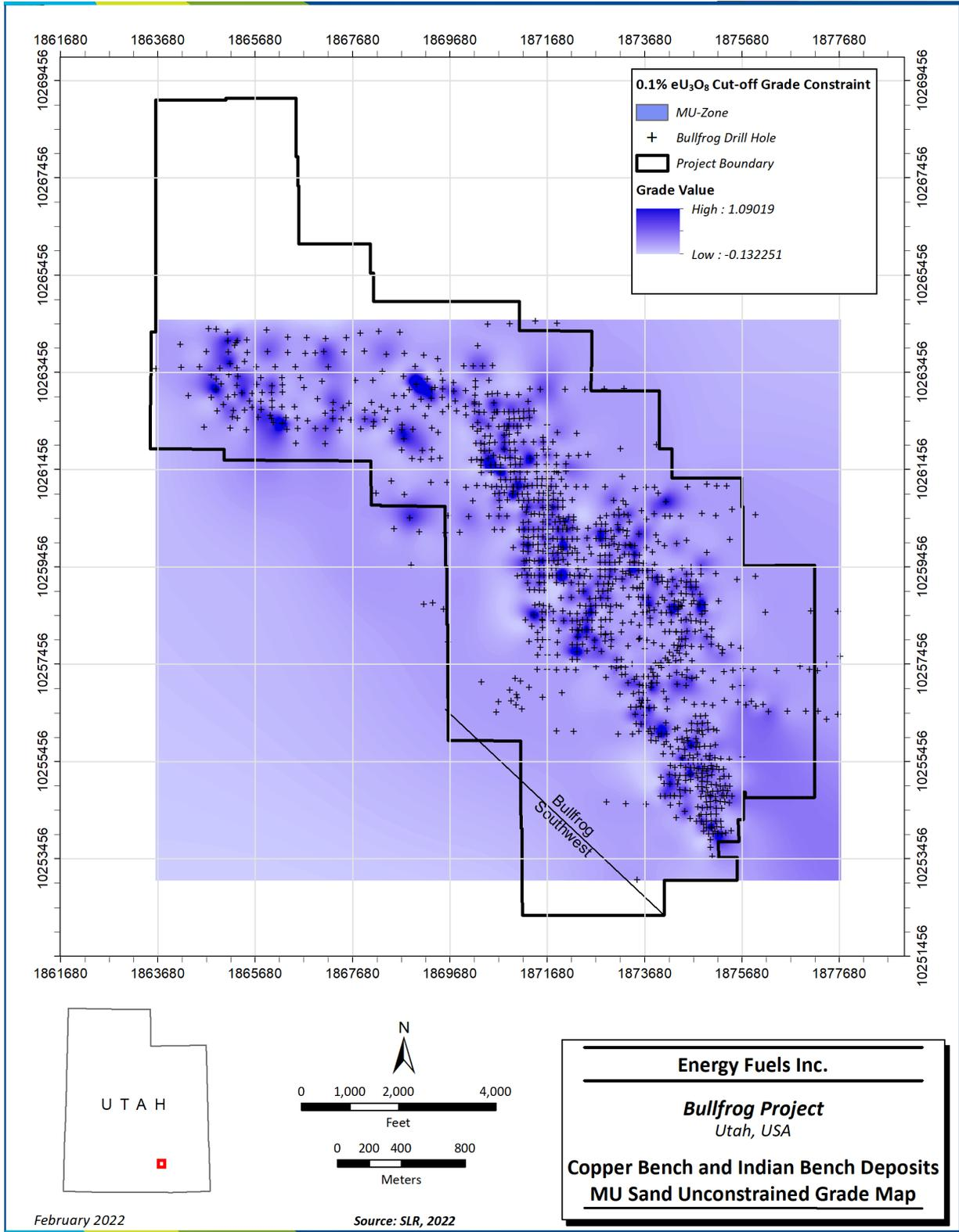
**Figure 14-5: Copper Bench and Indian Bench Deposits MU Sand Unconstrained Grade Map**
