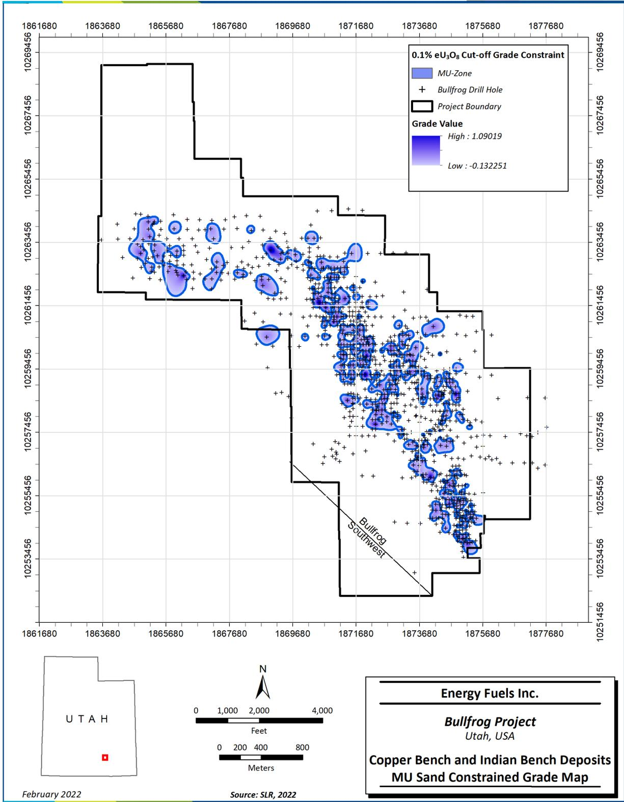
**Figure 14-8: Copper Bench and Indian Bench Deposits MU Sand Constrained Grade Map**
